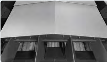
Enlarged chip ducts for smooth chip disposal
